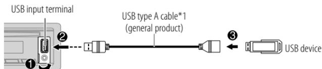
The source changes to USB automatically and playback starts.
