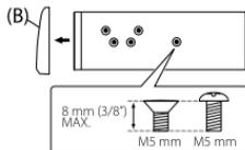
▲ Use only the specified screws. Using wrong screws might damage the unit.
