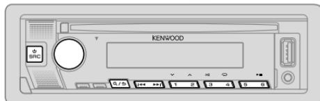
While in BT AUDIO source, you can connect to five Bluetooth audio devices and switch between these five devices.
